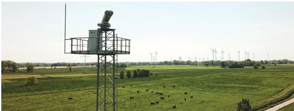
Figure 18 Terma 5002 Radar at a Wind Farm in Germany
