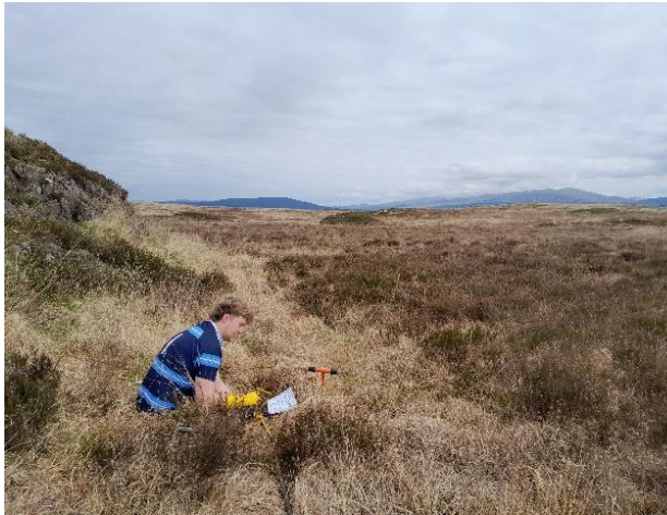
Photograph 3.1: Looking north from T3, at NGR 235616, 571956 (85 m AOD). Bedrock outcrop oriented north to south, abutting flat basin containing peat / organic soil. Peat depth nearby was 0.26 m. Slope gradients over the outcrop is gentle. No evidence of peat instability was noted. Moorland vegetation dominated by grasses and heather.
